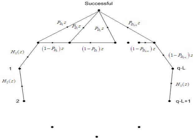
Fig. 3. Circular state diagram for the serial search acquisition system in multipath
