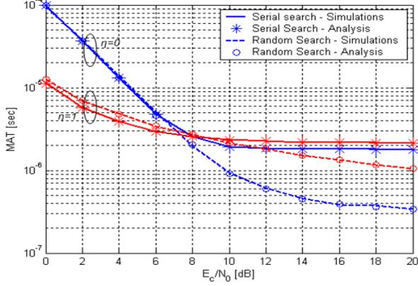
Fig. 4. Mean acquisition time in conventional multipath channel:  $L=16$
