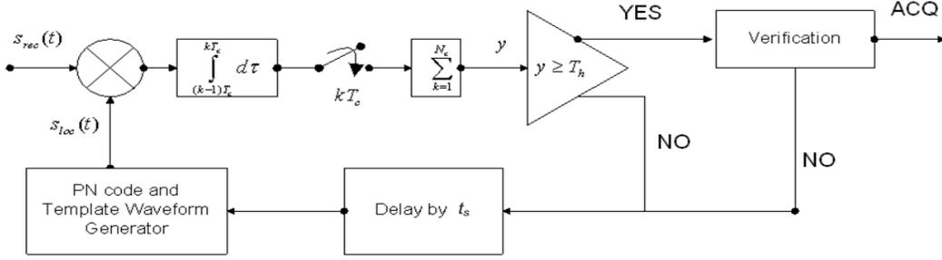
Fig. 1. Structure of an acquisition receiver employing serial search
